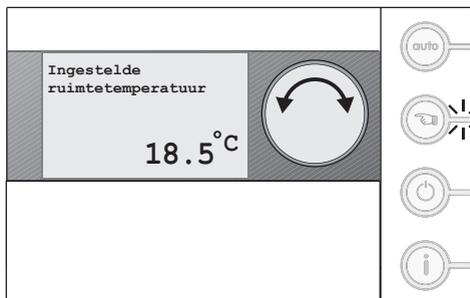
Fig. 4 Change temperature - manual operation
