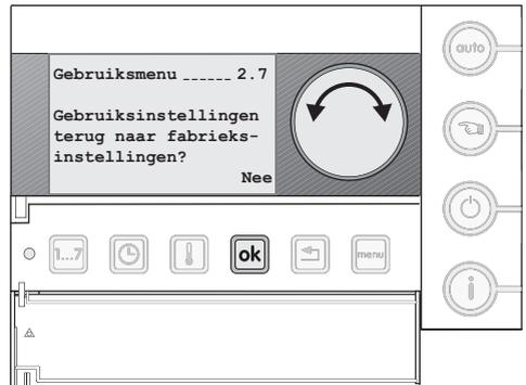
Fig. 35 Reset factory setting
