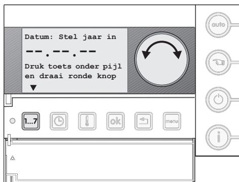
Fig. 19 Set-up date and time
