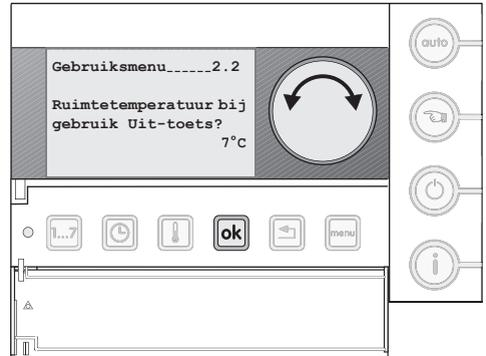
Fig. 30 Room temperature at off-function
