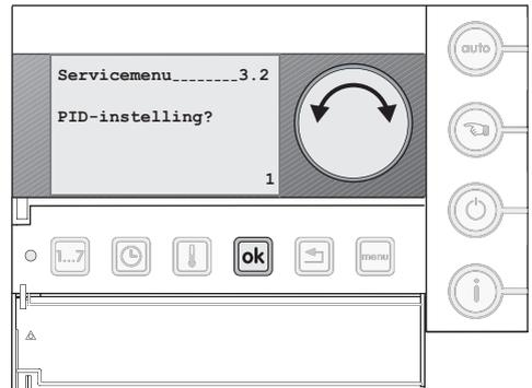
Fig. 39 PID-setting
