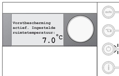
Fig. 5 De-activating the central heating
