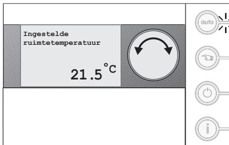
Fig. 3 Change temperature - auto-operation
