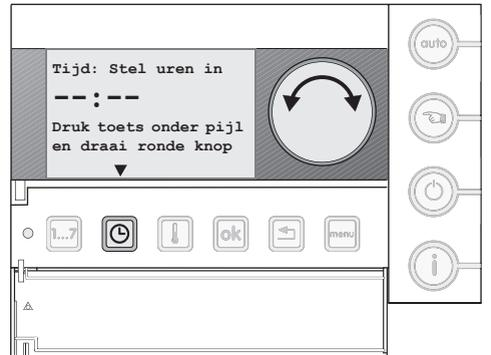
Fig. 7 Set-up time
