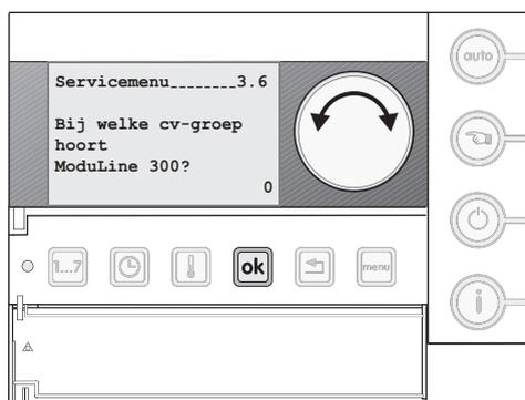
Fig. 43 Set-up heating circuit
