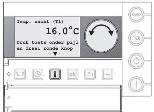
Fig. 8 Set-up temperature levels
