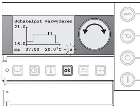
Fig. 27 Remove switching point
