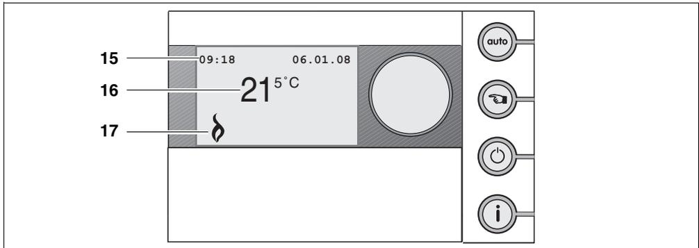
Fig. 2 Standard display ModuLine 300
