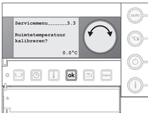
Fig. 40 Calibrate room temperature
