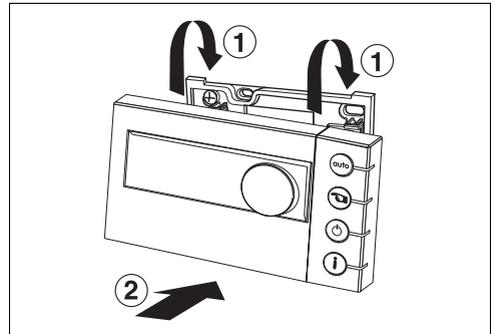
Fig. 17 Lock the thermostat into place
